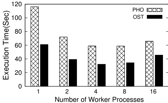
Figure 13: A comparison on the throughput of MapReduce servers based on Ostrich and Phoenix with the number of worker processes from 1 to 16. The workload has 100 mixed MapReduce jobs, which are randomly generated from our four benchmarks with about 100 Mbytes input.
