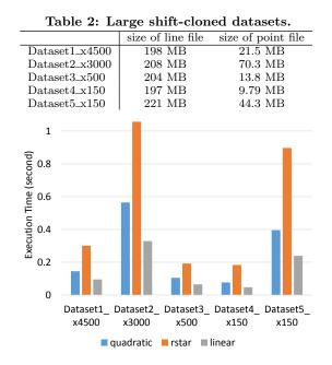
Figure 4: R-Tree building time (s) with different node splitting policies.
