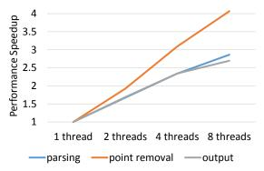
Figure 9: Parallel computation speedup for input parsing, point removal and output stages
