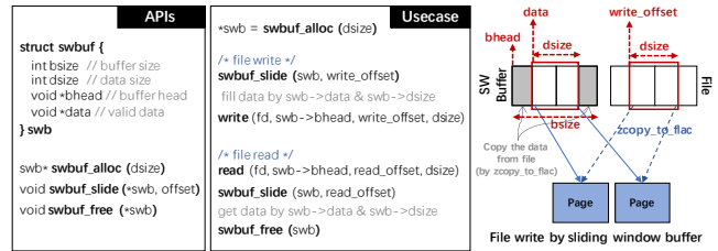
Figure 4: Sliding Window (SW) Buffer. Application uses SW buffer to serve page unaligned read/write. The sliding window is used to identify valid data in the buffer.
