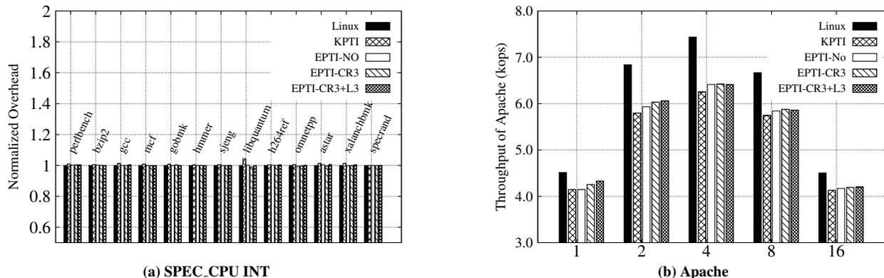
Figure 6: Figure (a) shows the overhead of all INT applications in SPEC\_CPU 2006 benchmark, lower the better. Figure (b) shows the throughput of Apache with different number of clients, higher the better.
