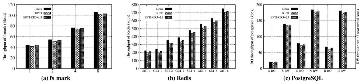
Figure 7: Figure (a) shows the throughput of fs\_mark with different threads. Figure (b) shows the throughput of SET and GET operations of Redis with different threads used by the client. Figure (c) shows the throughput of PostgreSQL under different workloads of RO (read-only) and RW (read-write) transactions. Higher the better.
