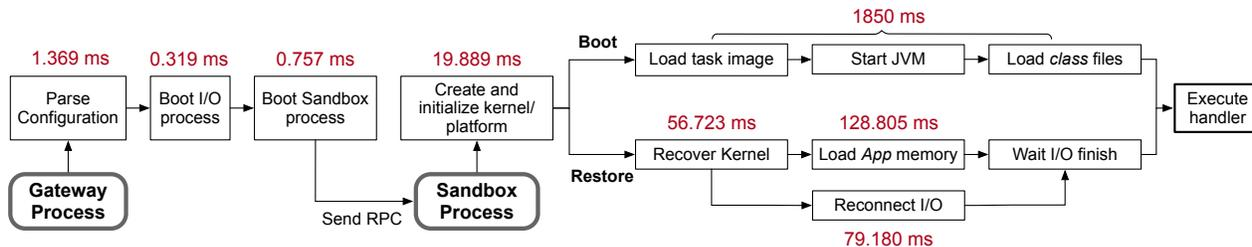
**Figure 2. Boot process of gVisor.** The numbers are the latency of each step of Java SPECjbb. The *Restore* path is the process of restoring a sandbox from a checkpoint image in gVisor (gVisor-restore).
