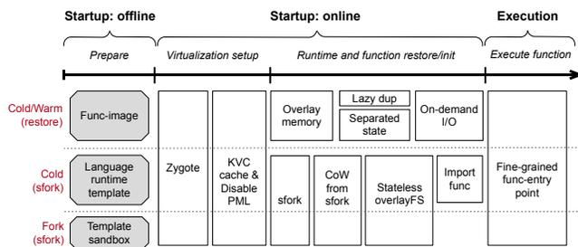
**Figure 10. Techniques/Optimizations used in Catalyzer for different kinds of boot.** Besides techniques introduced in §3 and §4, Catalyzer has other optimizations like the fine-grained func-entry point to further reduce startup latency.
