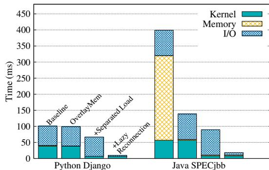
Figure 12. Breakdown of Catalyzer (*cold boot*) on gVisor.
