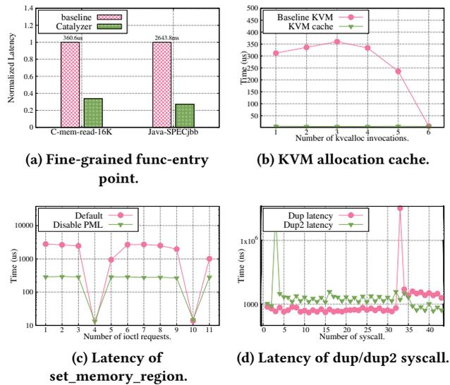
**Figure 16. Optimizations in Catalyzer.** Figure (a) shows fine-grained func-entry point can reduce the execution latency by 3x. From Figure (b), adding a cache in KVM can reduce the latency of `kvccallc`. Figure (c) shows the latency of `set_memory_region` `ioctl` in KVM and disabling PML achieves 10x shorter latency. Figure (d) shows the latency of `dup` syscall during boot. The burst one takes about 30 ms for the syscall.
