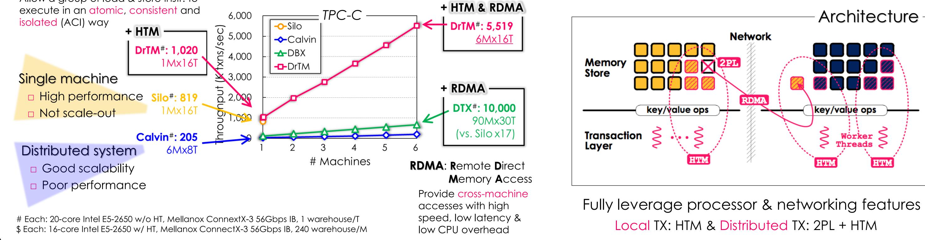
**DrTM**: In-memory TX processing system Target: OLTP workloads Two independent components: Transaction layer & memory store A partitioned global address space
