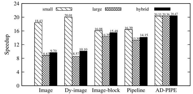
Fig. 17. The hyper-threading performance of SURF parallelism on various image sets.
