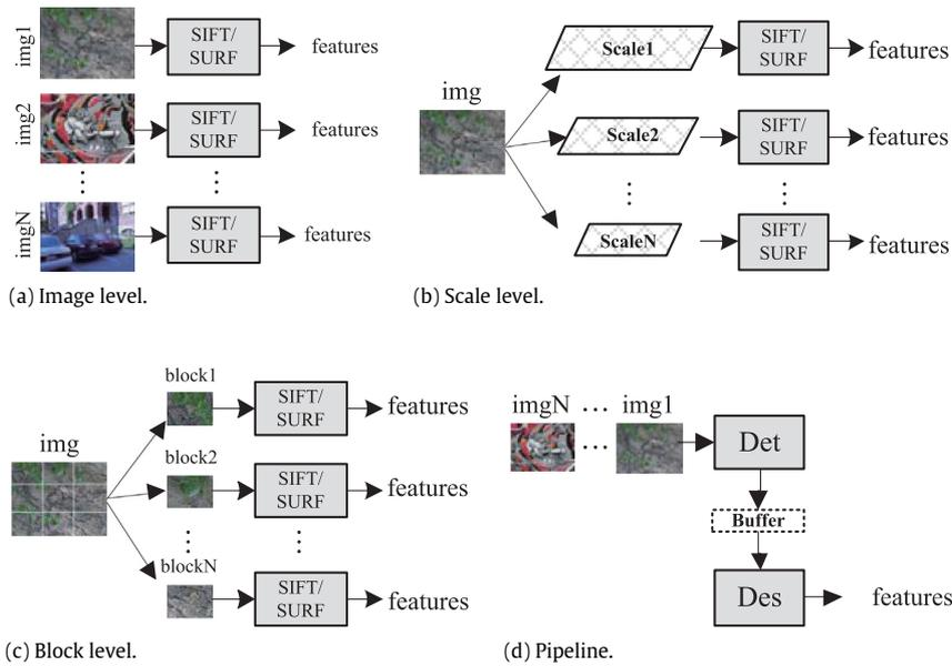
Fig. 3. Different primary parallelism in the LFAs (SIFT and SURF). Blocks with shadow are those components mapped on different cores.
