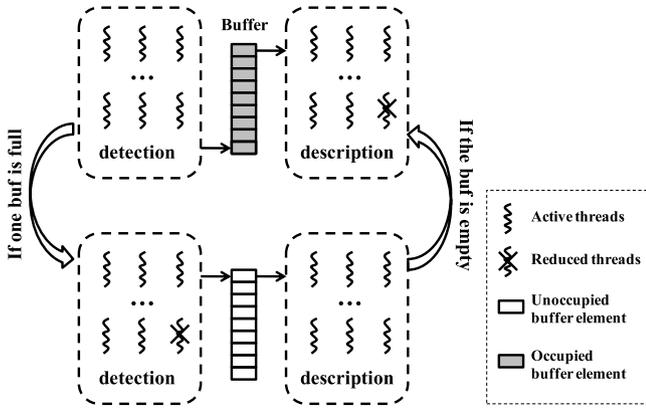
Fig. 9. The basic architecture of AD-PIPE.
