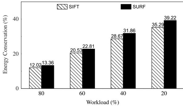
**Fig. 20.** The energy conservation performance of AE-PIPE for constant workloads when energy consumption of idle CPU is 40% of the normal state.
