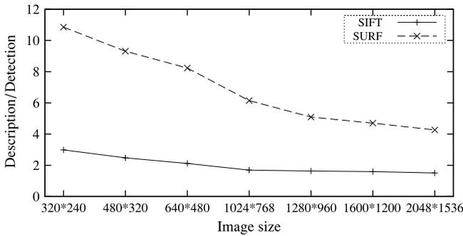
Fig. 4. Time distributions between detection and description stages. The ratio is the time of description stage dividing that of detection stage.
