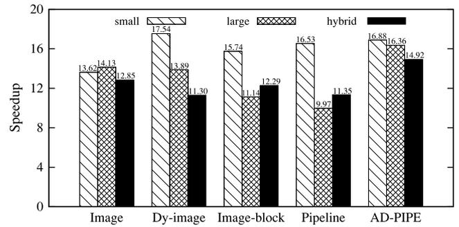
Fig. 16. The hyper-threading performance of SIFT parallelism on various image sets with 16 physical cores.
