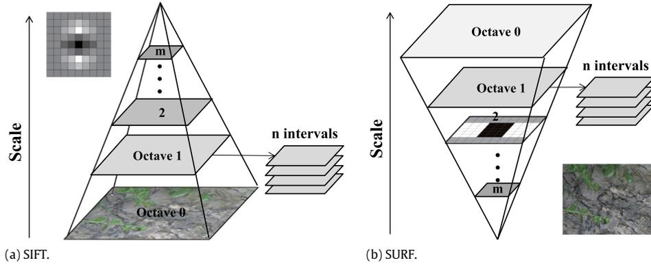
Fig. 2. The pyramid structure in SIFT and SURF. The pyramid consists of  $m$  octaves; each octave consists of  $n$  intervals.
