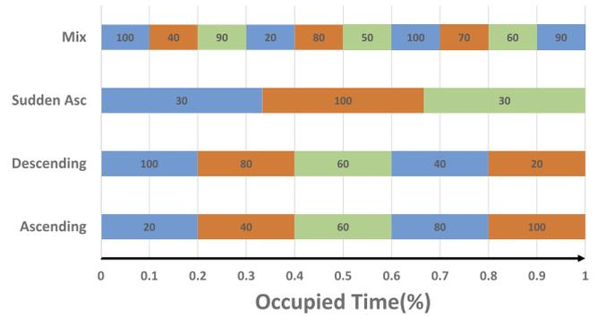
**Fig. 21.** Four practical workloads we are testing. The width of a single block means the percentage of occupied time in the whole test and the number in the block means the percentage of input workloads.
