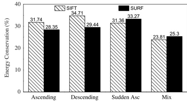
**Fig. 22.** The energy conservation performance of AE-PIPE for practical workloads when energy consumption of idle CPU is 10% of the normal state.
