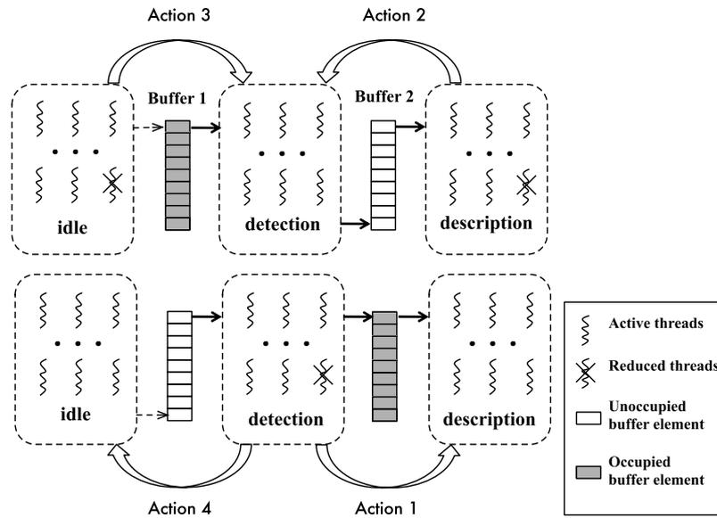
Fig. 11. Dynamic scheduling of AE-PIPE threads.
