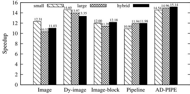
Fig. 15. The speedup of various SURF parallelism for different image sets on 16 cores.
