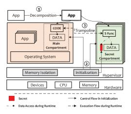
Figure 1: Architecture overview of SeCage
