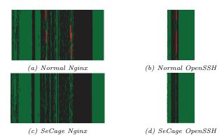
Figure 8: Heap memory layout for Nginx and OpenSSH server processes. (Green blocks are memory in use, black areas are unused and the red bars are targeted *secrets* found in the memory.)
