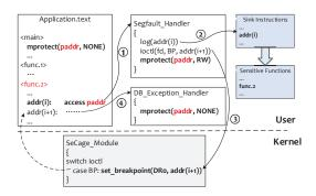
Figure 7: Combining mprotect and debug exception to dynamically extract sink instructions
