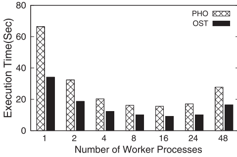
Fig. 23. A comparison on the throughput of MapReduce servers based on Ostrich and Phoenix with the number of worker processes from 1 to 48. The workload has 100 mixed MapReduce jobs, which are randomly generated from our four benchmarks with about 100MByte input.
