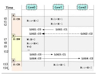
**Figure 2.** An overview of the CREW protocol based on MMU protection: left squares are a shared object in different states: concurrent-read (CR) and exclusive-write (EW); top squrares are CPU cores accessing the shared object. The solid arrows indicate the captured "happen-before" relationship between two memory operations. Log2 is a redundant log and LOG3 is an overcontrained log.
